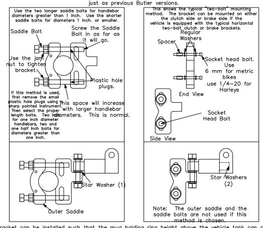
This bracket can be installed such that the mug holding ring height above the vehicle tank can change. Here are some examples.
